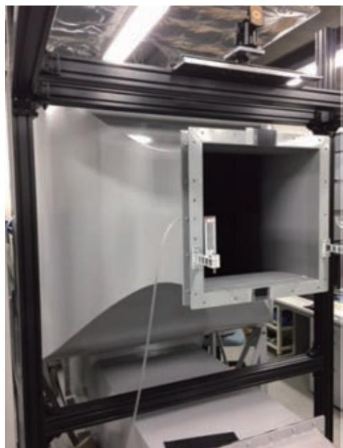
Wind tunnel equipment with  $400 \times 400$  mm outlet
