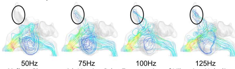
Airflow Changes with Varying Inlet Frequencies of Vibrating Nebulizer
