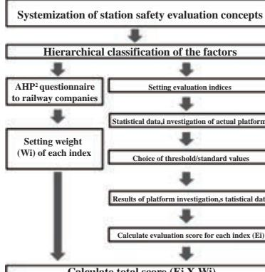
Fig. 2. Flow of safety evaluation score calculation steps
