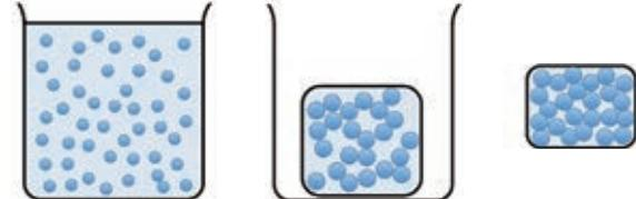
Adjusting Metal Oxide Film by Sol-Gel Method
