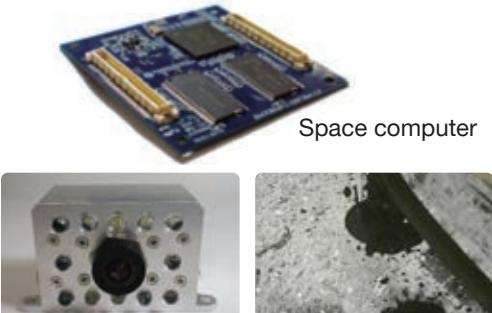
Camera installed in Hayabusa2 (left) and an image of the touchdown (right)
