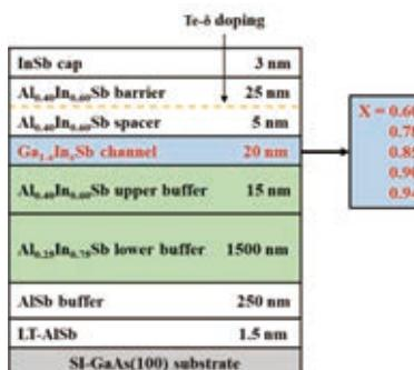
Layered structure of GaInSb quantum well channels using step buffers.
