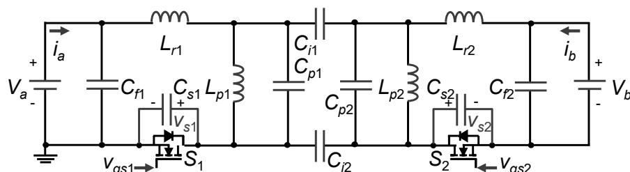
Load-independent class E<sup>2</sup> parallel resonant DC-DC converter (with capacitor coupler)
