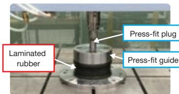
Press-fitting of a foam metal plug
