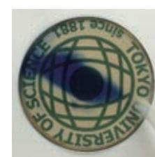
Only a portion sprayed with hydrogen gas is colored.
