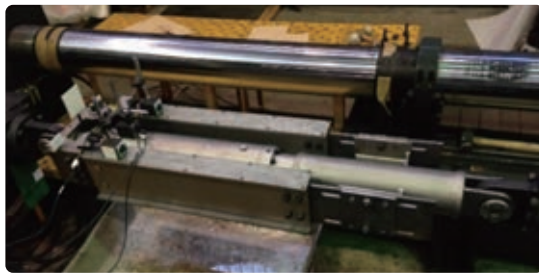
Oil damper with a spring as a test body
