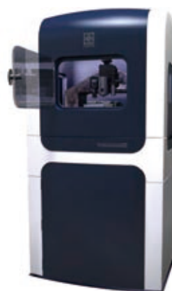
Analysis/interpretation: shape measurement, nano-property evaluation (SPM), adsorption property (QCM), wettability evaluation and various surface analyses
