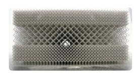
Modeling of a lattice structure by exploiting the characteristics of a metal 3D printer
