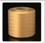
High-strength aramid fiber (para-aramid fiber)
