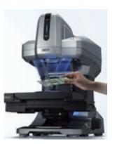
Analysis/interpretation: shape measurement, nano-property evaluation (SPM), adsorption property (QCM), wettability evaluation and various surface analyses
