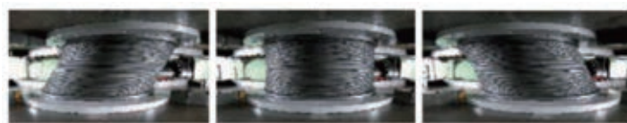
Compression shear test of laminated rubber
