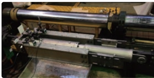
Oil damper with a spring as a test body
