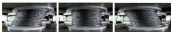
Compression shear test of laminated rubber
