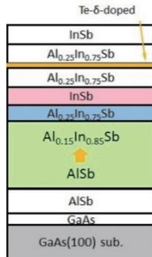
Layer structure of an InSb quantum well channel for which the electron mobility has been increased by strain control
