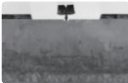
Cross-sectional TEM image of the prototype strain-controlled InSb HEMT (gate electrode length: 80 nm)
