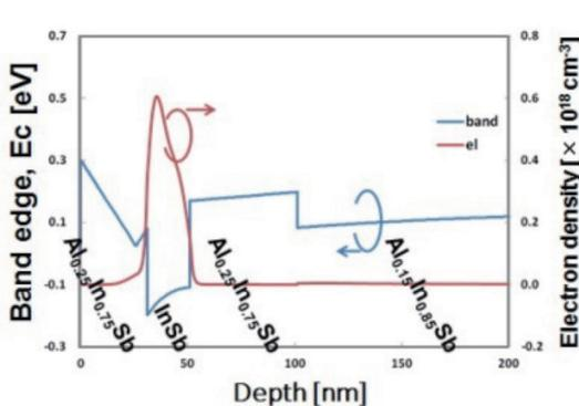
Simulation results for the band structure and electron density distribution of the strain-controlled InSb HEMT
