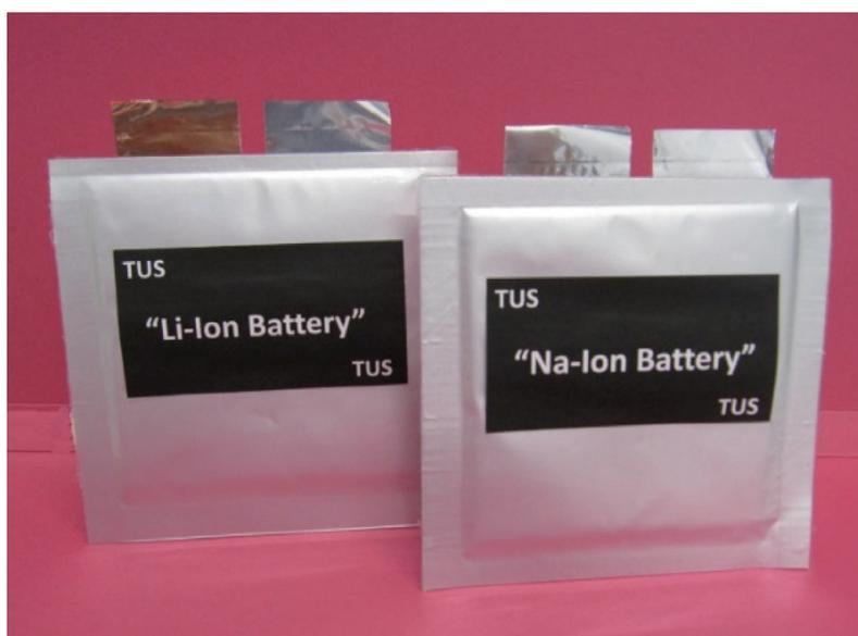
Our laboratory developed a 3 V-class Na-ion battery that uses  $\text{Na}[\text{Ni}_{1/2}\text{Mn}_{1/2}]\text{O}_2$  as the positive electrode and hard carbon as the negative electrode. This battery is capable of operating at room temperature without any hazards and its energy density has reached 60–80% that of widely used graphite/LiCoO<sub>2</sub> batteries.
