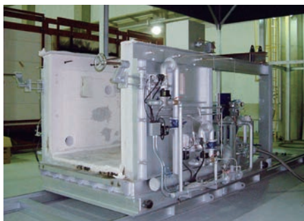
Structural Fire Testing Furnace (Medium scale)
