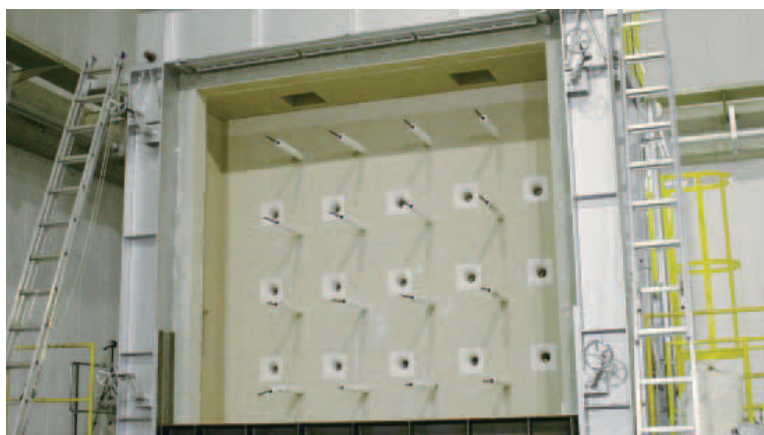
Structural fire testing furnace (large-scale, for walls)
