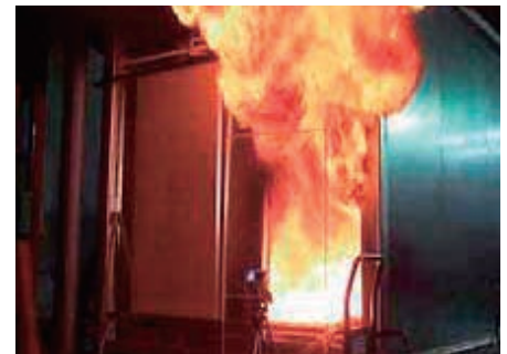
Room Corner Testing Unit (ISO 9705)
