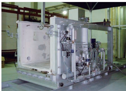
Structural Fire Testing Furnace (Medium scale)
