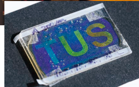
Cellulose liquid crystal elastomer films change color when stretched with force.
